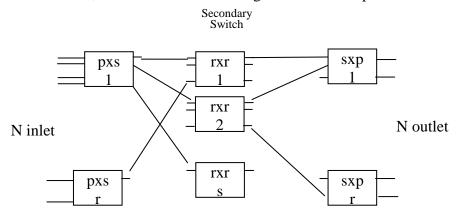
In a two stage network the blocking probability is:  $P_B=[a+(1-a)b]^g$  where a are incoming links and b outgoing links here a=b=N $P_B=[N+(1-N)N]^g$  In a three stage network the blocking probability is:
